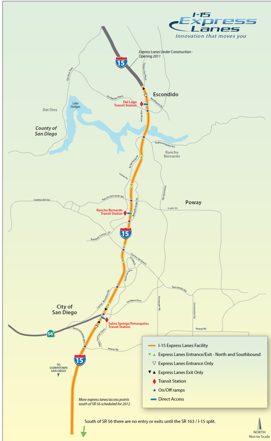
Figure 6: I-15 Corridor Map Showing 20-mile I-15 Express Lanes (from the split at I-15 and SR 163 to SR 78 in Escondido) (Fastrak, 2012)
