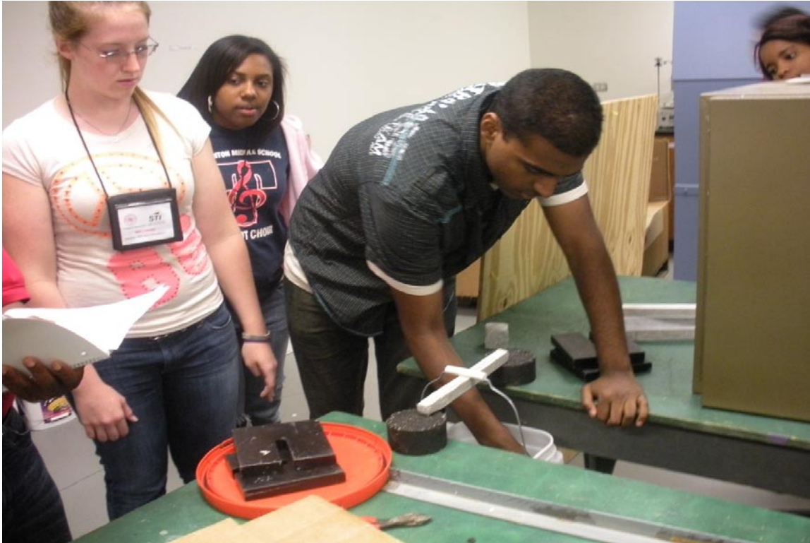
Group 1 adding weights to a bucket to test the strength of their concrete beam
