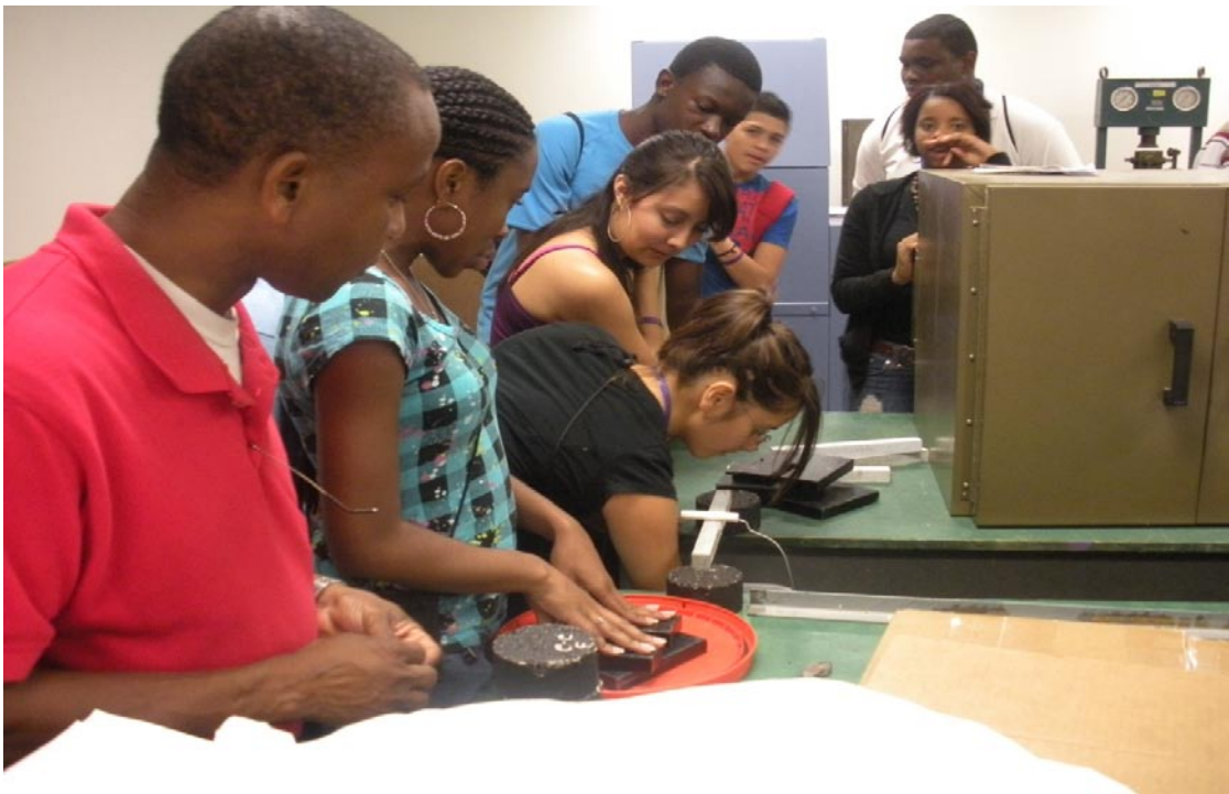
Group 3 adding weights to a bucket to test the strength of their concrete beam
