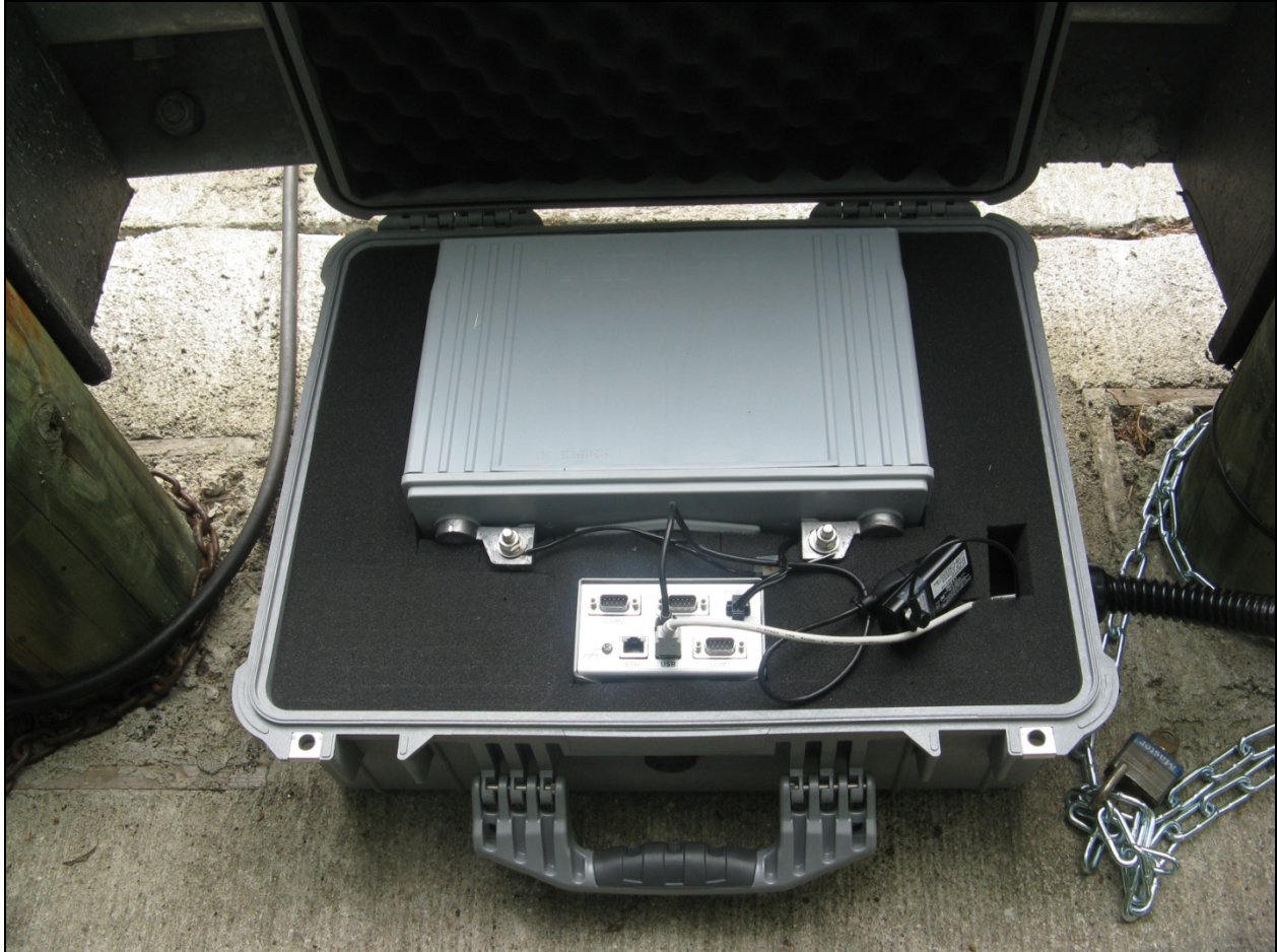
Figure 13. Portable Bluetooth Travel Time Monitoring Equipment Configuration
