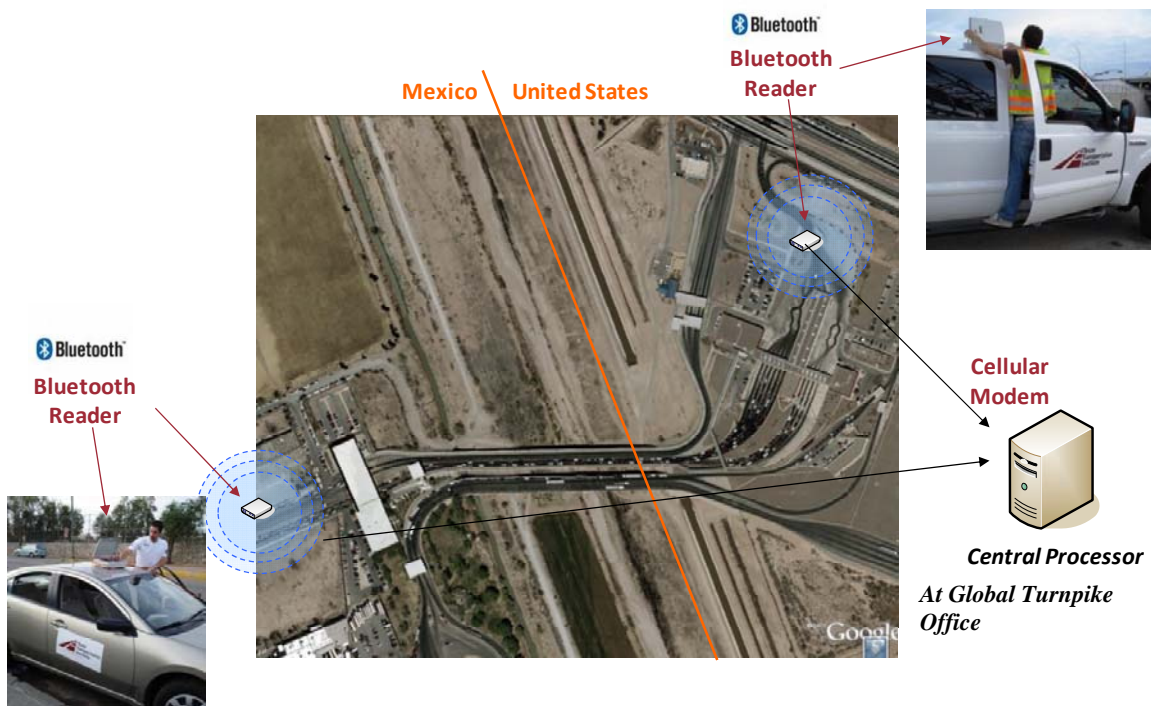
Figure 57. A Typical Setup of Bluetooth Readers at U.S. and Mexico Sides of the Border.
