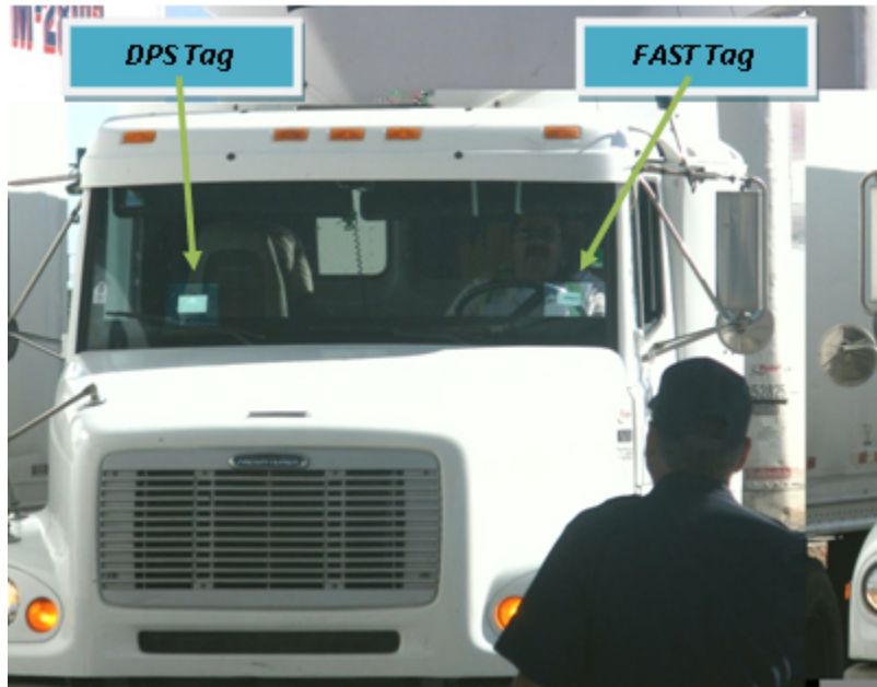
Figure 48. A Truck Carrying both DPS and CBP Issued RFID Tags.
